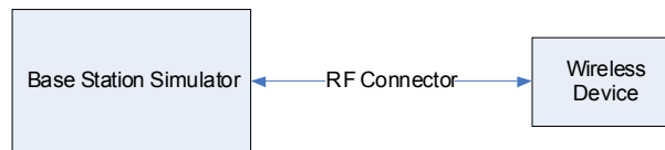
Figure 9-3 Power Measurement Setup
