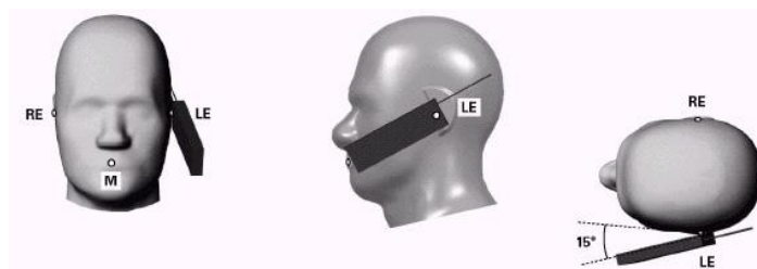
Figure 6 Front, Side and Top View of Ear/15° Tilt Position
