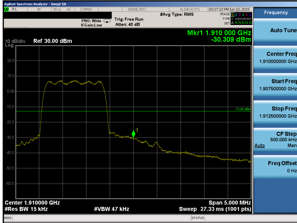
Plot 6-75. Band Edge Plot (PCS CDMA Mode – Ch. 1175)
