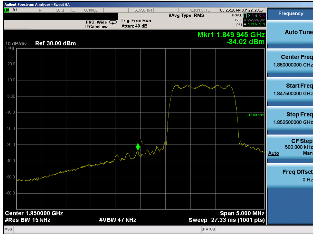
Plot 6-73. Band Edge Plot (PCS CDMA Mode – Ch. 25)
