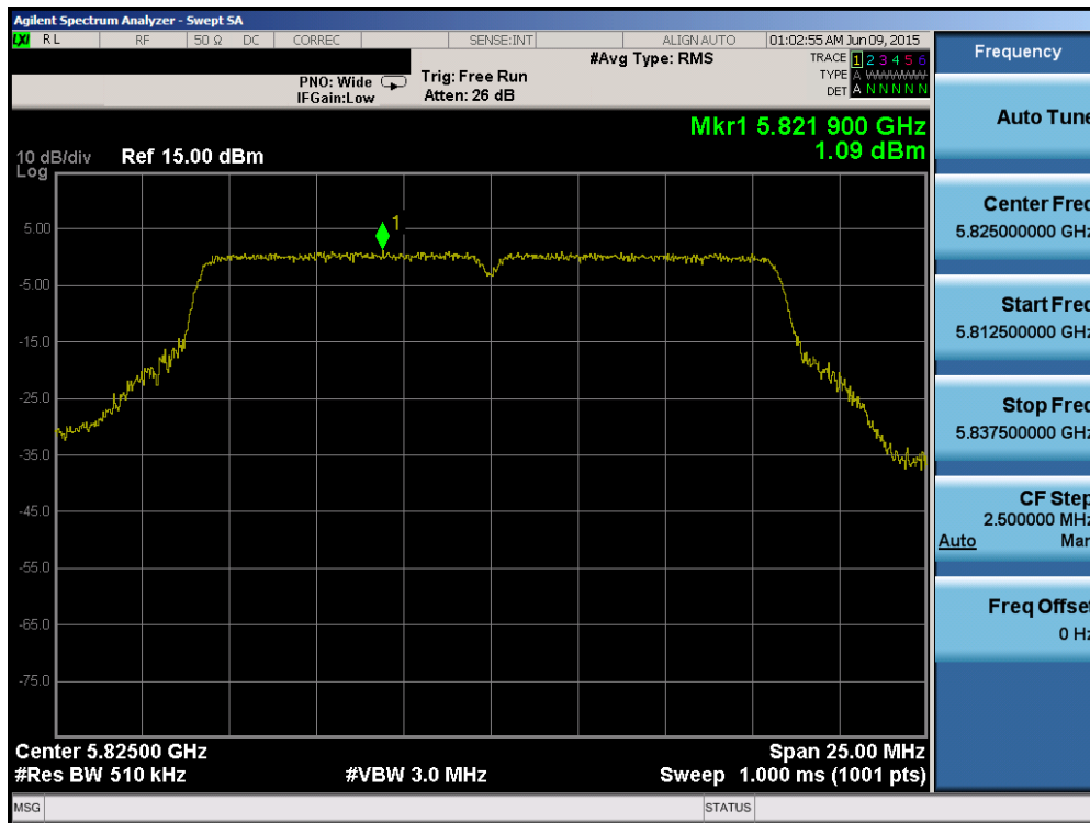
Plot 6-108. Power Spectral Density Plot (802.11a (UNII Band 3) – Ch. 165)
