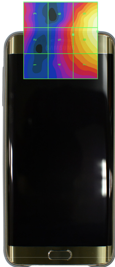
Figure 15-4 E-Field WD Scan overlay
