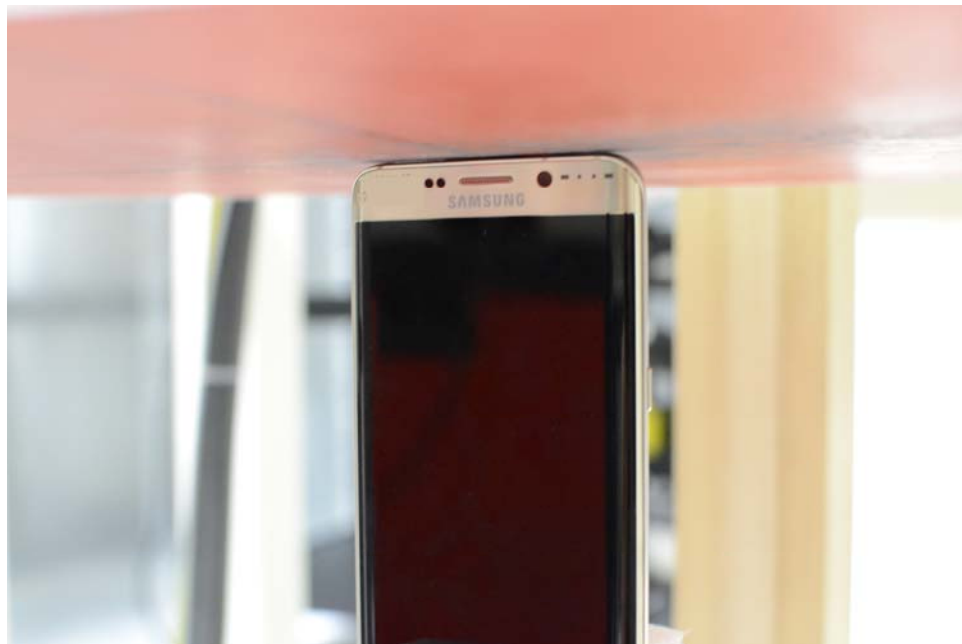
SAR Test Setup Photo 12– Top Edge at 0.0 cm (Extremity)
