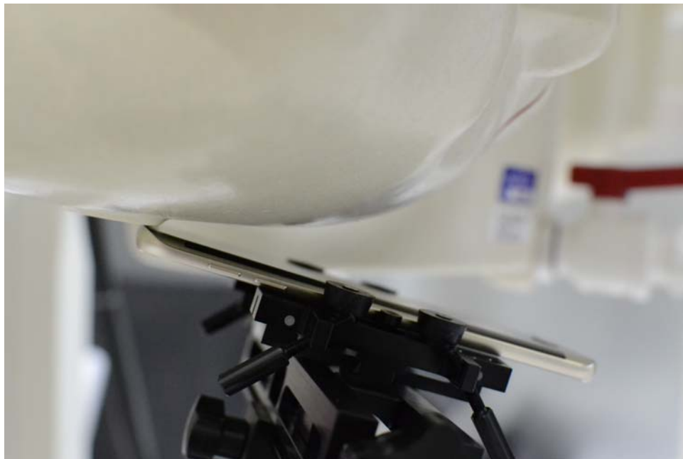
SAR Test Setup Photo 2- Right Tilt
