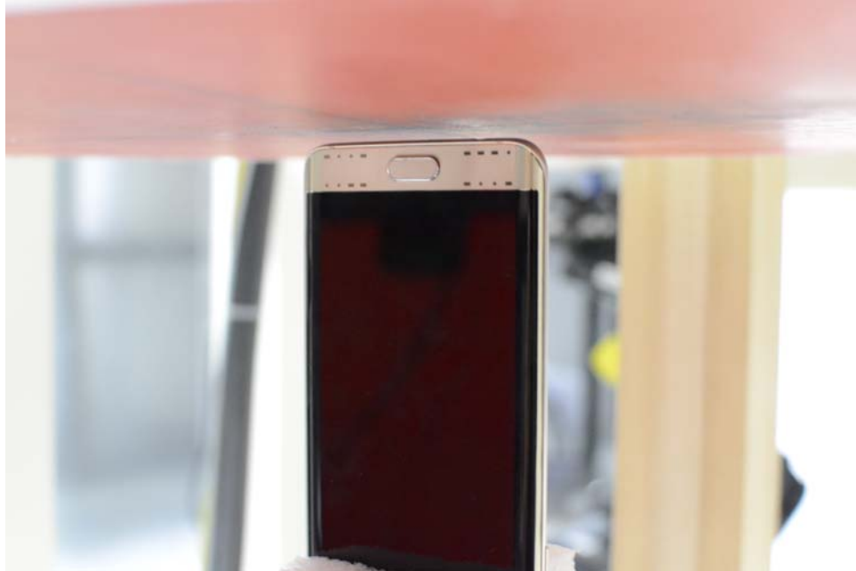
SAR Test Setup Photo 15– Bottom Edge at 0.3 cm (Extremity)
