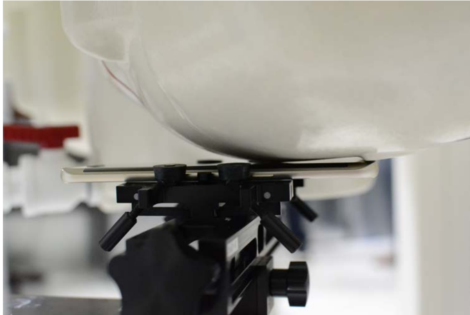
SAR Test Setup Photo 3- Left Cheek
