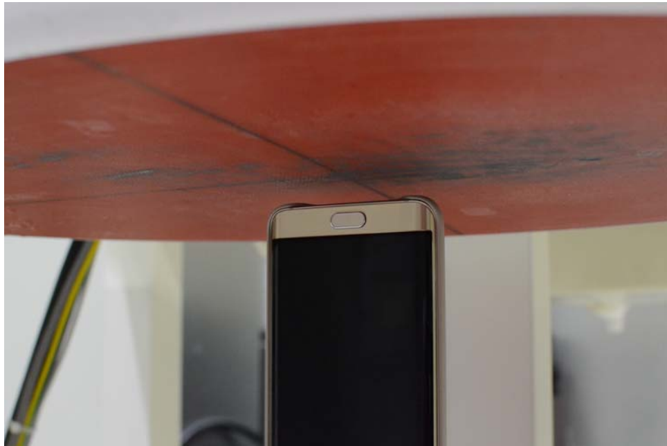
SAR Test Setup Photo 10: Bottom Edge at 1.0 with Wireless Charging Cover
