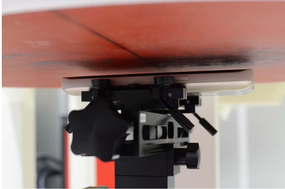
SAR Test Setup Photo 7: Front Side at 1.0 cm with Wireless Charging Cover
