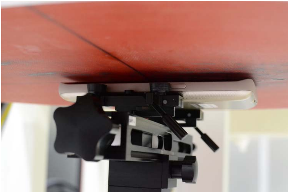
SAR Test Setup Photo 8: Front Side at 0.1 cm with Wireless Charging Cover
