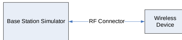
Figure 9-2 Power Measurement Setup
