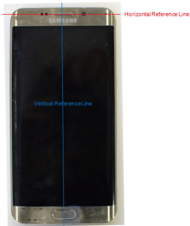
SAR Test Setup Photo 21– DUT Reference Lines
