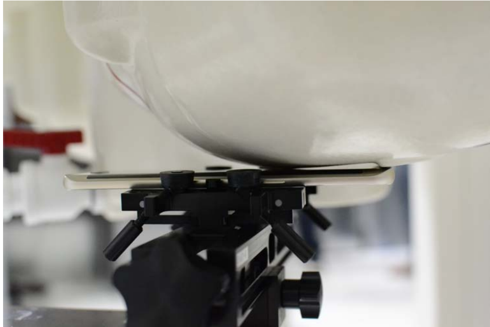
SAR Test Setup Photo 3– Left Cheek
