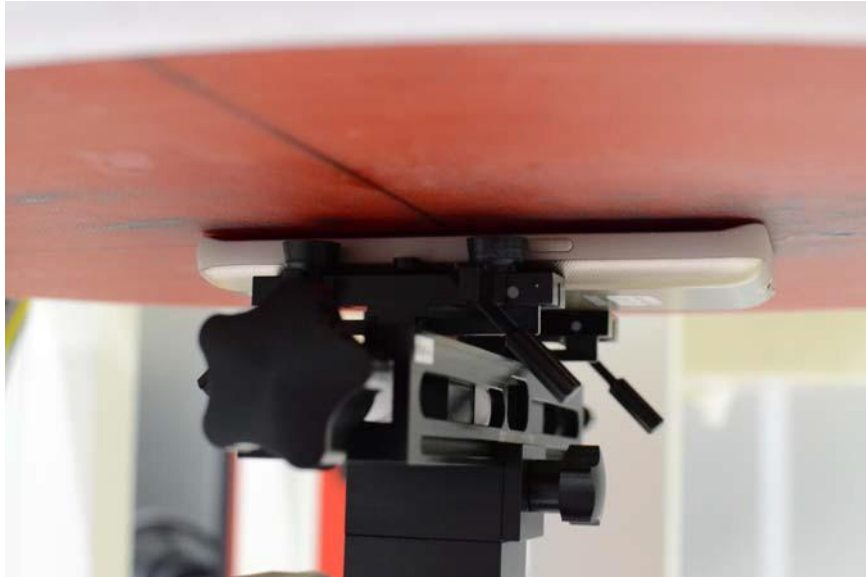
SAR Test Setup Photo 5 — Front Side at 0.0 cm (Phablet)
