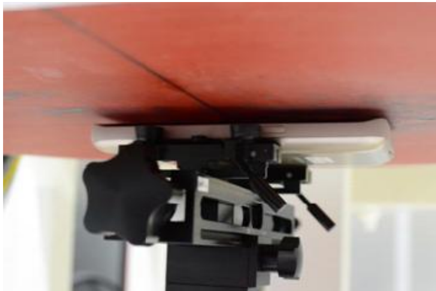
SAR Test Setup Photo 6— Front Side at 0.1 cm (Phablet)
