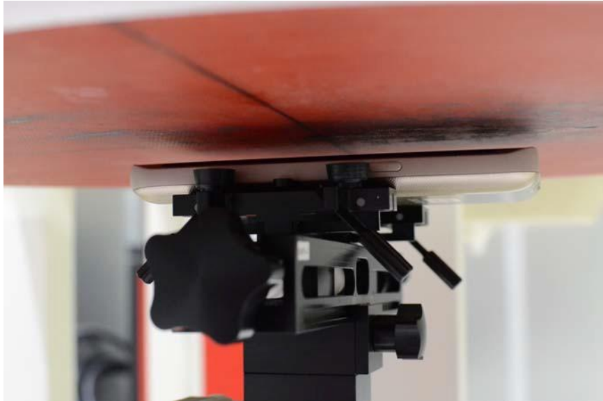
SAR Test Setup Photo 7 - Front Side at 1.0 cm (Hotspot)
