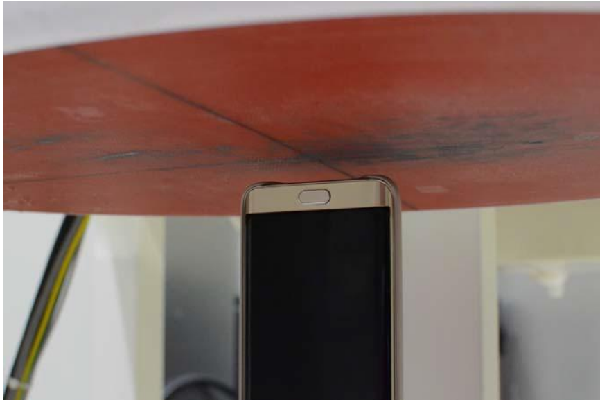
SAR Test Setup Photo 9 – Bottom Edge at 1.0 cm (Hotspot)
