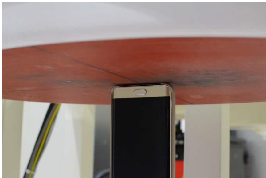
SAR Test Setup Photo 8 – Bottom Edge at 0.0 cm (Phablet)
