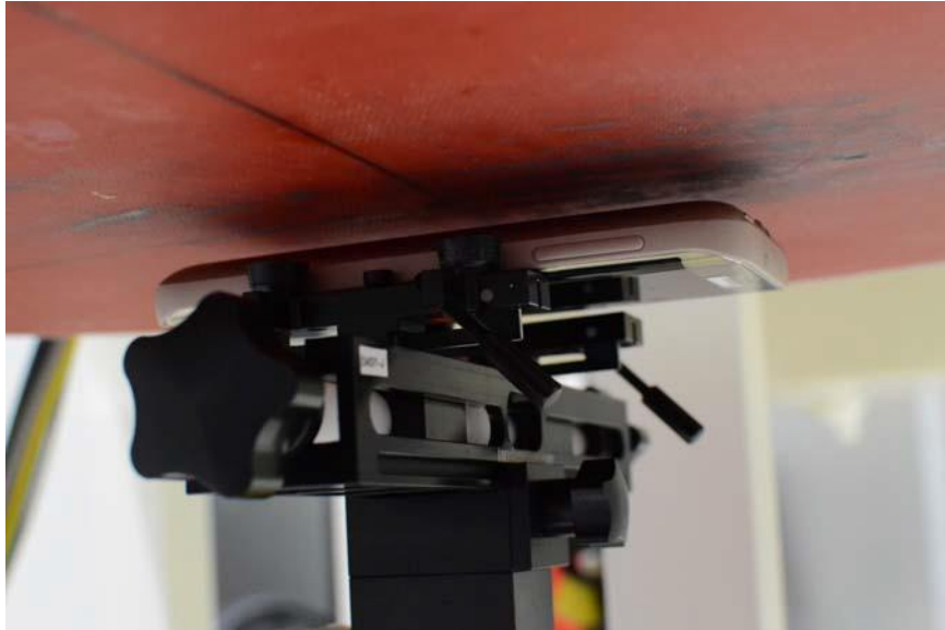
SAR Test Setup Photo 3 – Back Side at 1.0 cm (Hotspot)
