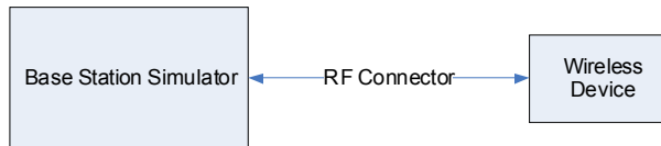
Figure 9-3 Power Measurement Setup
