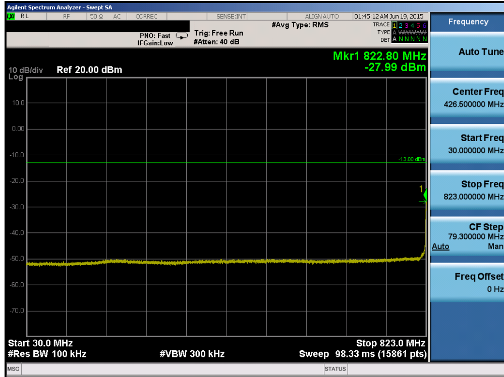
Plot 6-26. Conducted Spurious Plot (Cellular WCDMA Mode – Ch. 4132)
