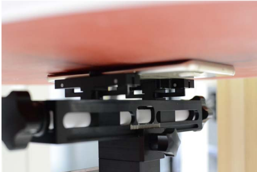
SAR Test Setup Photo 16: Front at 0 mm
