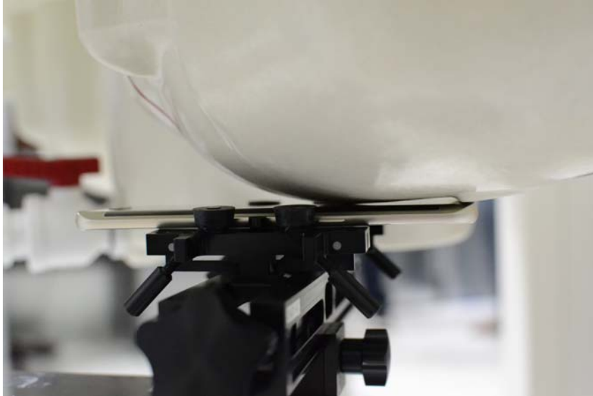
SAR Test Setup Photo 3: Left Cheek
