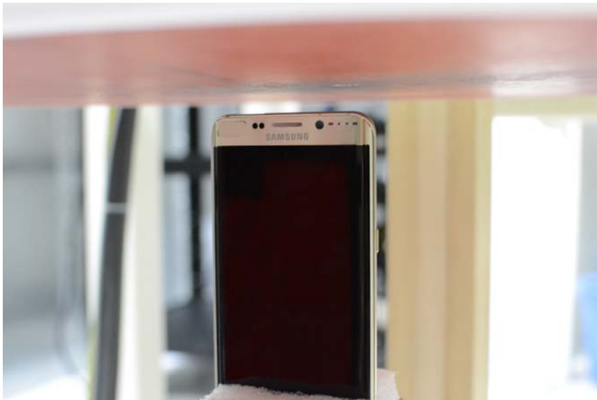
SAR Test Setup Photo 8: Top at 10 mm
