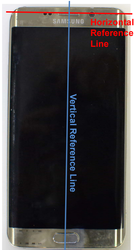
SAR Test Setup Photo 21: Horizontal and Vertical Reference Lines
