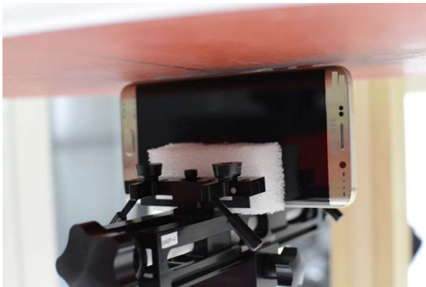
SAR Test Setup Photo 20: Left at 0 mm
