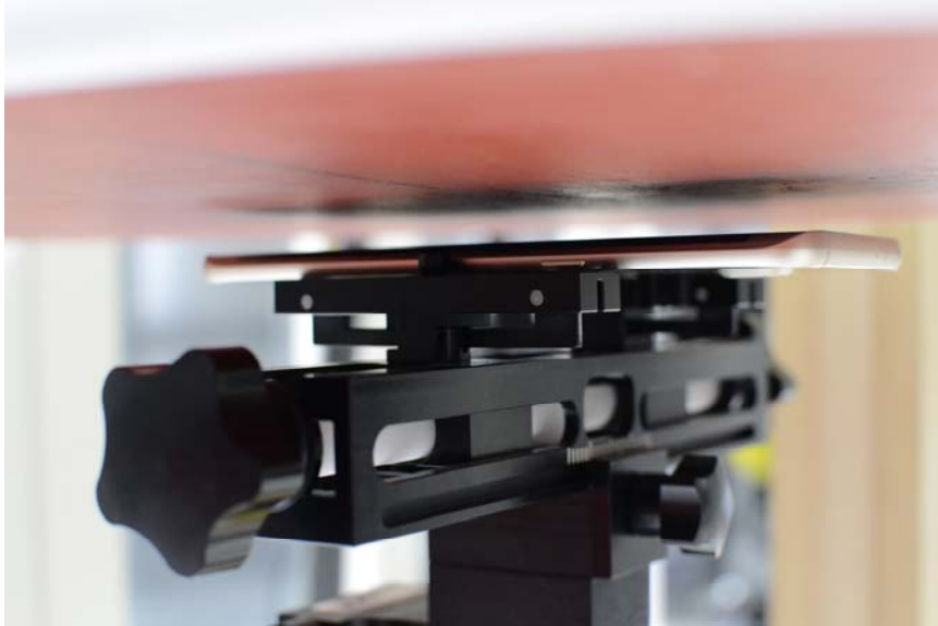
SAR Test Setup Photo 7: Front at 10 mm
