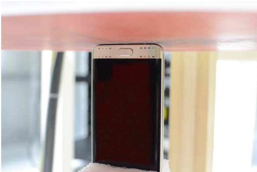
SAR Test Setup Photo 18: Bottom at 0 mm
