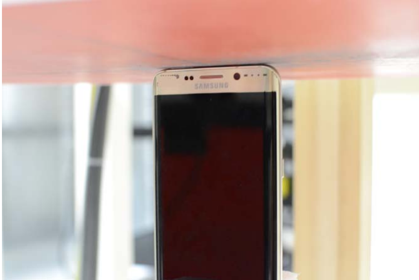
SAR Test Setup Photo 17: Top at 0 mm
