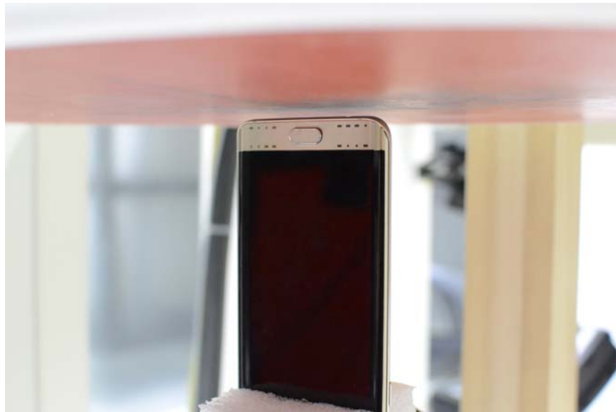
SAR Test Setup Photo 14: Bottom at 4 mm
