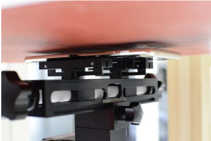
SAR Test Setup Photo 12: Back at 4 mm
