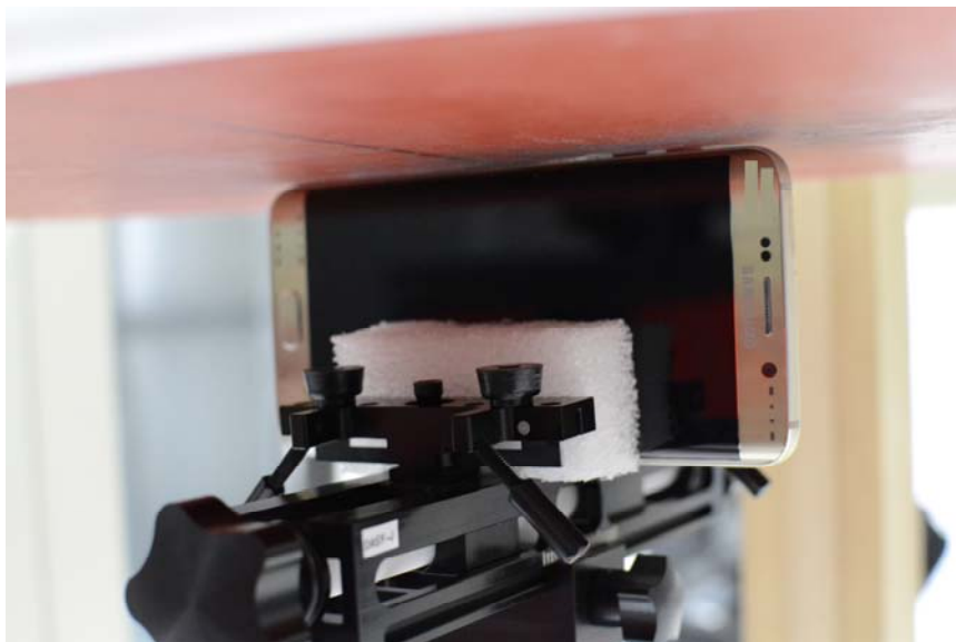
SAR Test Setup Photo 20: Left at 0 mm
