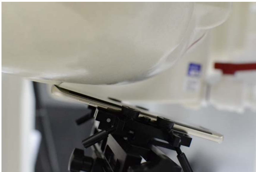
SAR Test Setup Photo 2: Right Tilt
