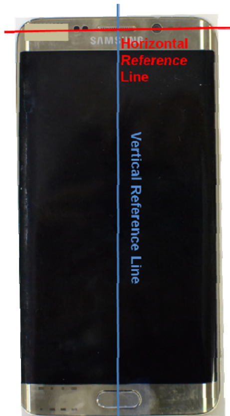
SAR Test Setup Photo 12 – DUT Reference Lines
