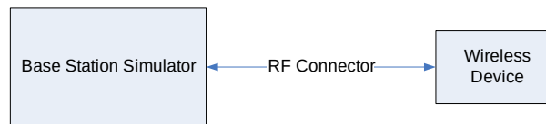
Figure 9-3 Power Measurement Setup
