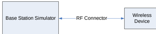
Figure 9-1 Power Measurement Setup
