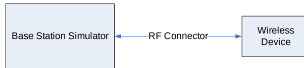
Figure 9-2 Power Measurement Setup
