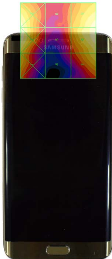
Figure 18-4 E-Field WD Scan overlay
