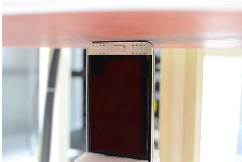
SAR Test Setup Photo 14– Bottom Edge at 0.0 cm (Extremity)
