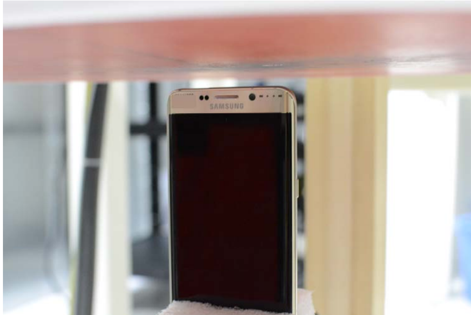
SAR Test Setup Photo 13– Top Edge at 1.0 cm (Hotspot)
