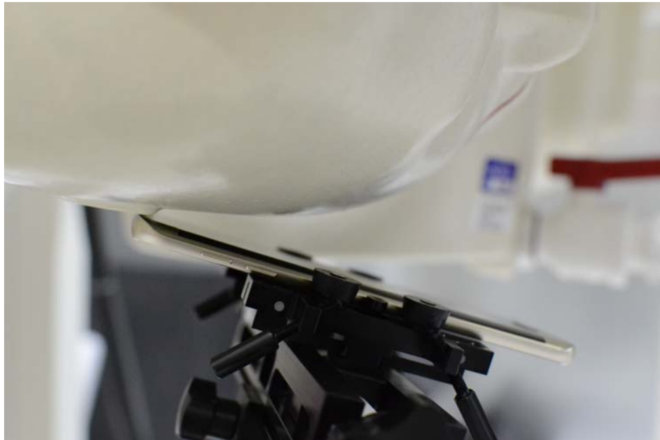
SAR Test Setup Photo 2- Right Tilt
