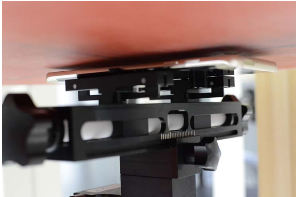
SAR Test Setup Photo 6– Back Side at 0.3 cm (Extremity)
