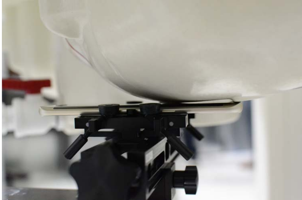
SAR Test Setup Photo 3– Left Cheek
