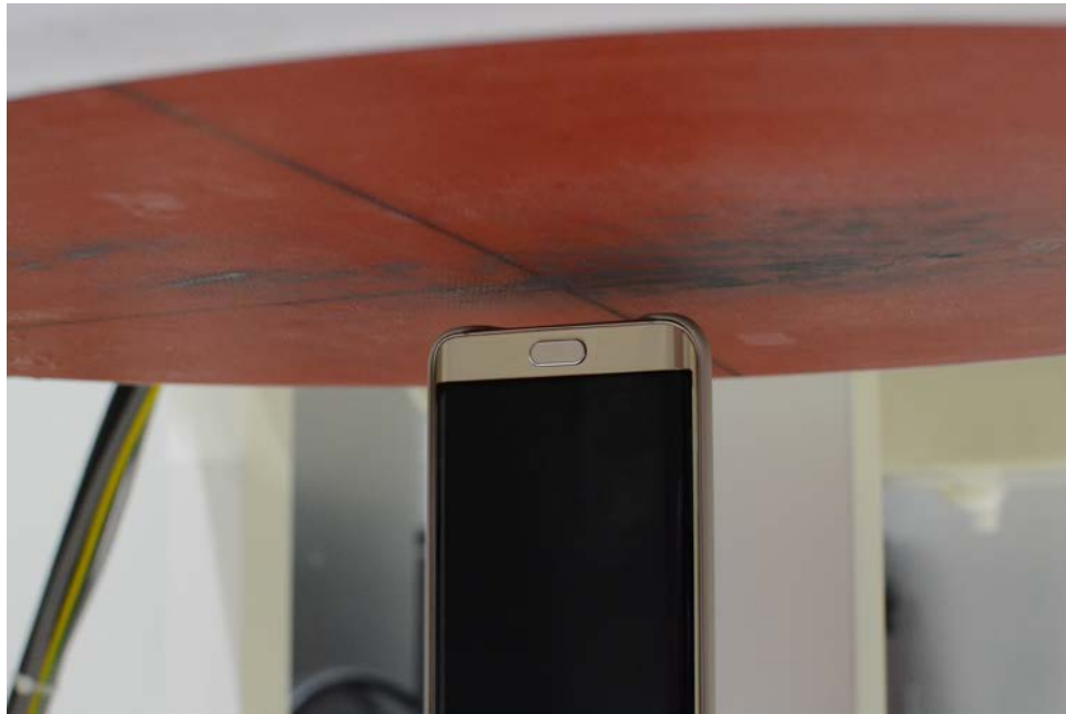
SAR Test Setup Photo 8 – Bottom Edge at 1.0 cm (Hotspot)
