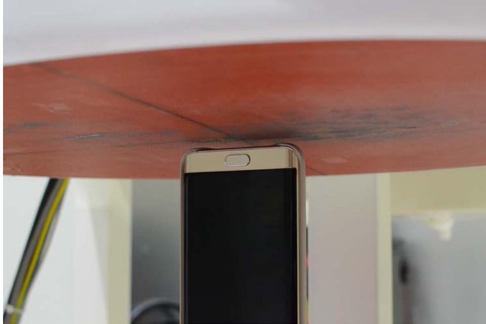
SAR Test Setup Photo 7 – Bottom Edge at 0.4 cm (Phablet)
