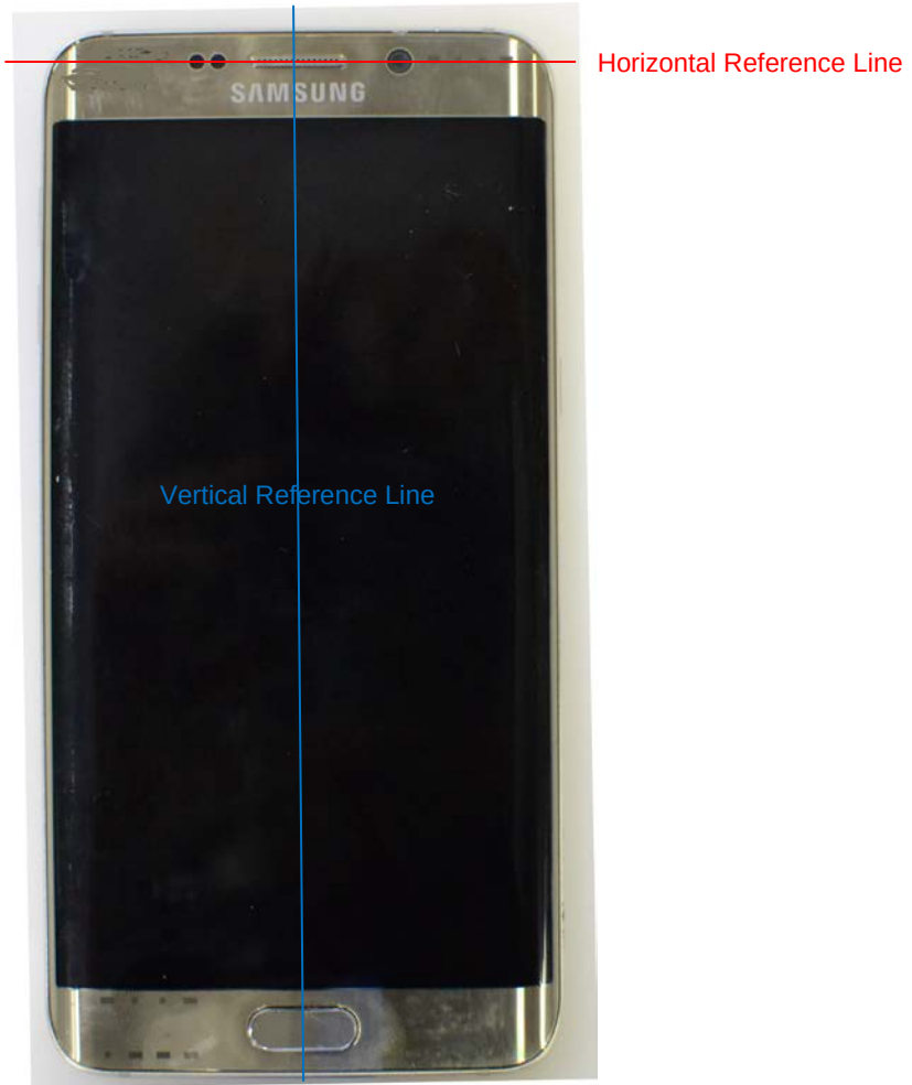
SAR Test Setup Photo 9 – DUT Reference Lines
