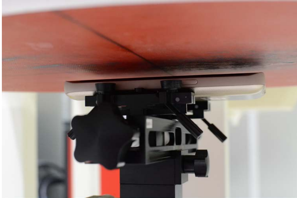
SAR Test Setup Photo 5 - Front Side at 1.0 cm (Hotspot)
