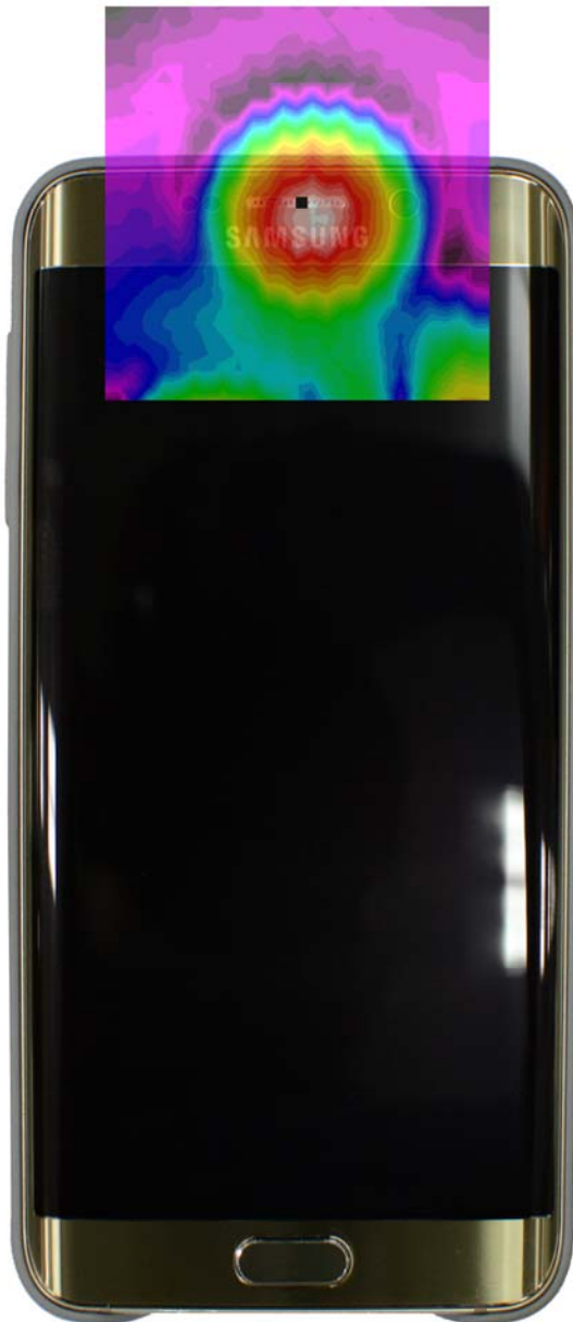
Figure 12-3 Axial T-coil Scan Overlay Magnetic Field Distributions
