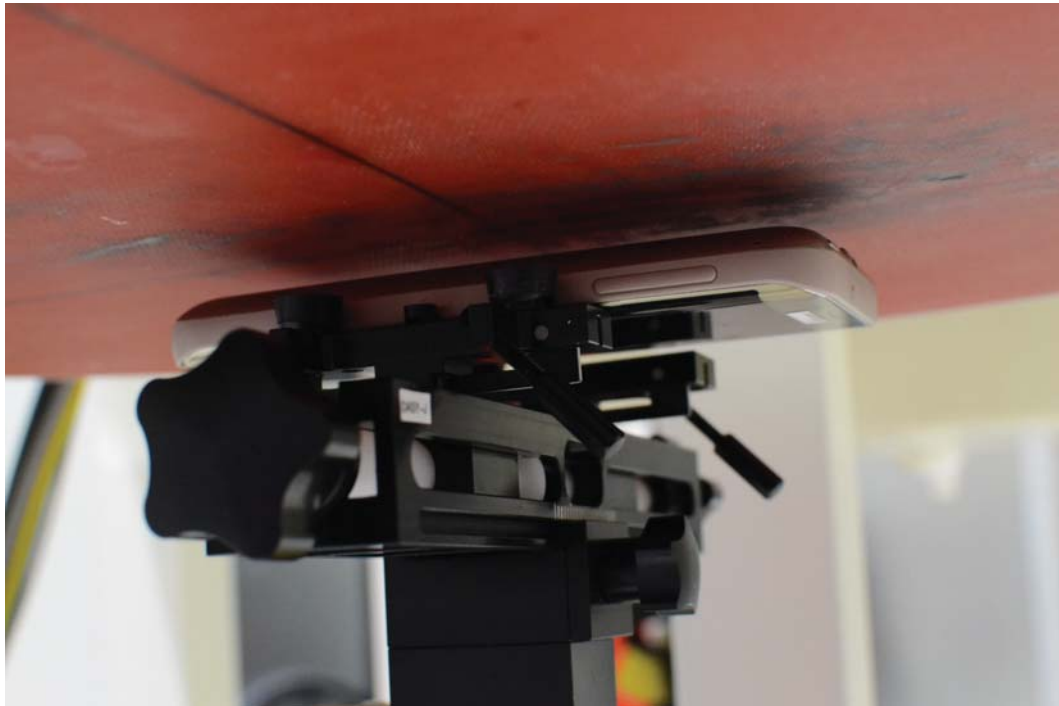
SAR Test Setup Photo 4 – Back Side at 1.0 cm (Hotspot)
