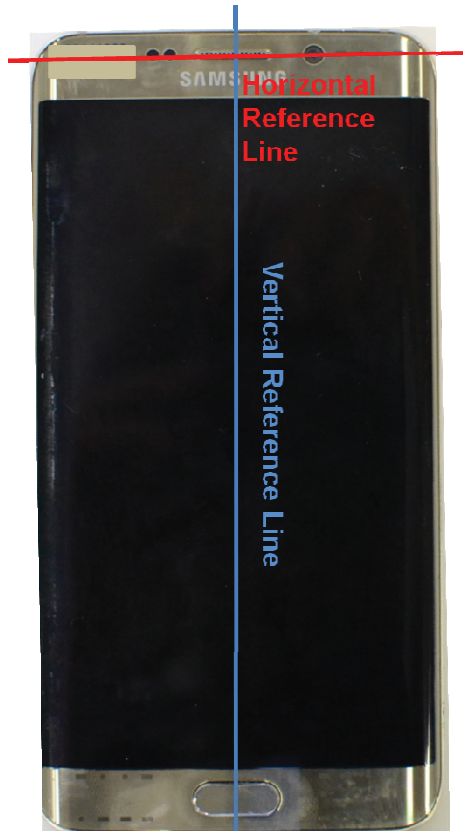
SAR Test Setup Photo 11 – DUT Reference Lines
