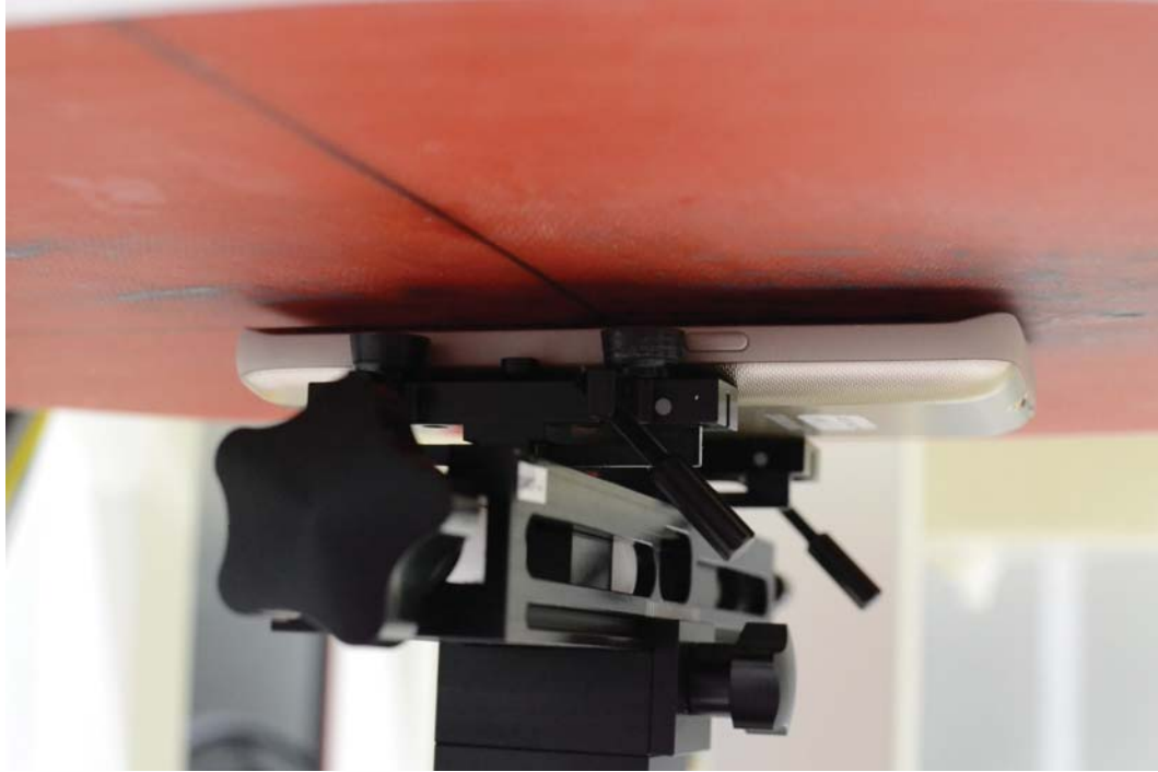
SAR Test Setup Photo 7 - Front Side at 0.4 cm (Phablet)
