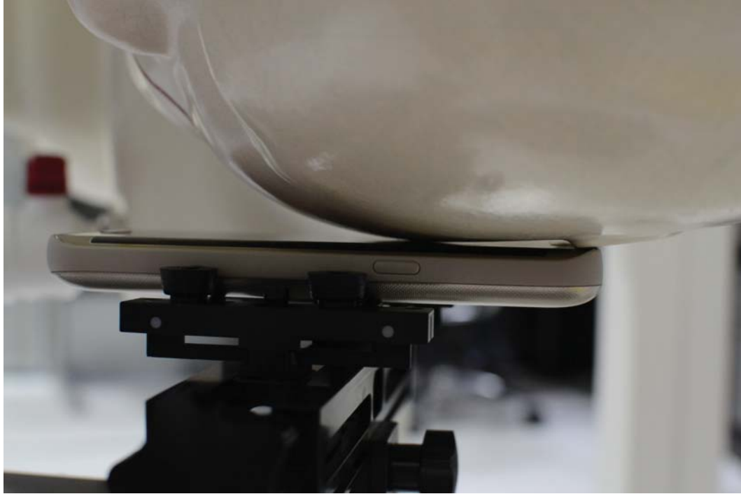
SAR Test Setup Photo 3 – Left Cheek
