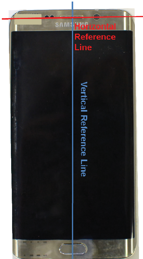
SAR Test Setup Photo 11 – DUT Reference Lines
