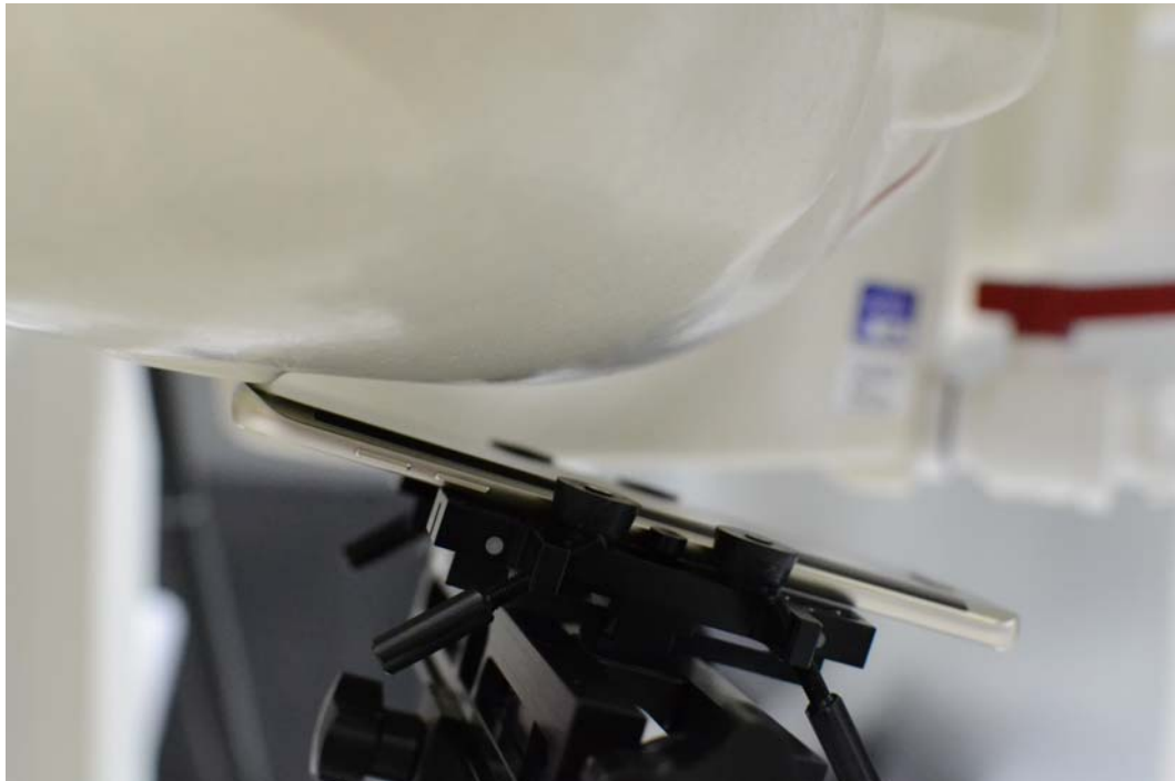
SAR Test Setup Photo 2- Right Tilt
