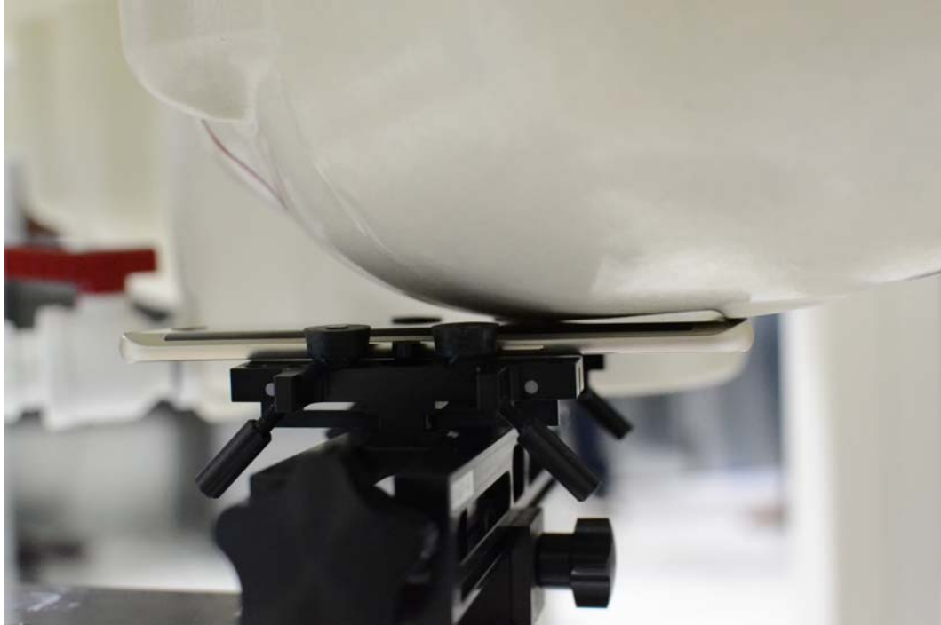
SAR Test Setup Photo 3– Left Cheek
