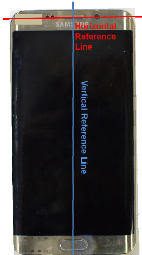
SAR Test Setup Photo 21 – DUT Reference Lines
