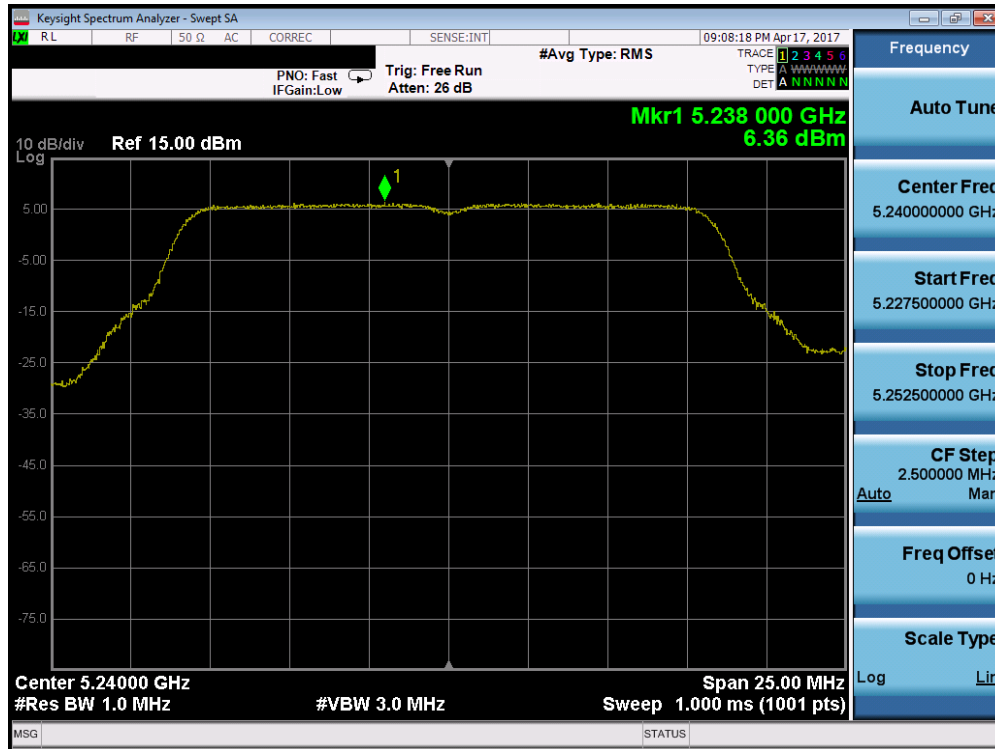
Plot 7-42. Power Spectral Density Plot (802.11a (UNII Band 1) – Ch. 48)
