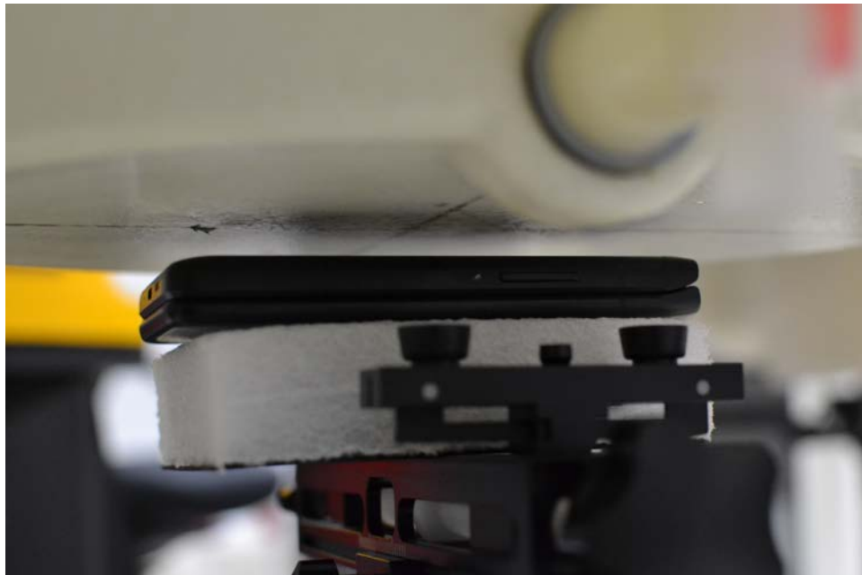
SAR Test Setup Photo 10 – Back Side at 10 mm
