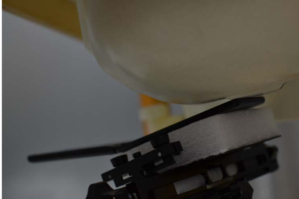
SAR Test Setup Photo 7 – Left Tilt
