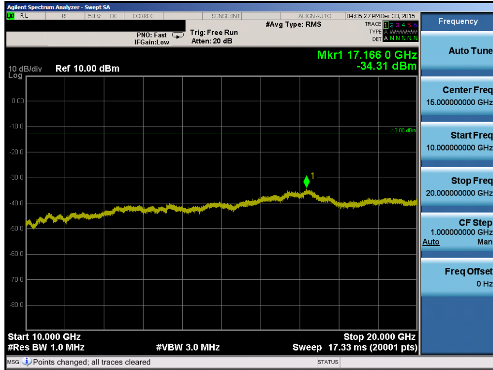
Plot 7-39. Conducted Spurious Plot (PCS WCDMA Mode – Ch. 9400)
