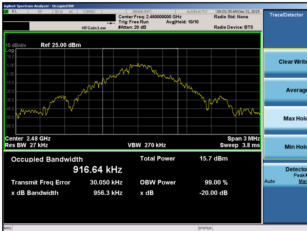
Plot 7-3. 20dB Bandwidth Plot (Bluetooth, 1Mbps – Ch. 78)
