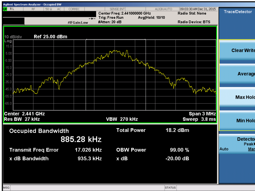
Plot 7-2. 20dB Bandwidth Plot (Bluetooth, 1Mbps – Ch. 39)
