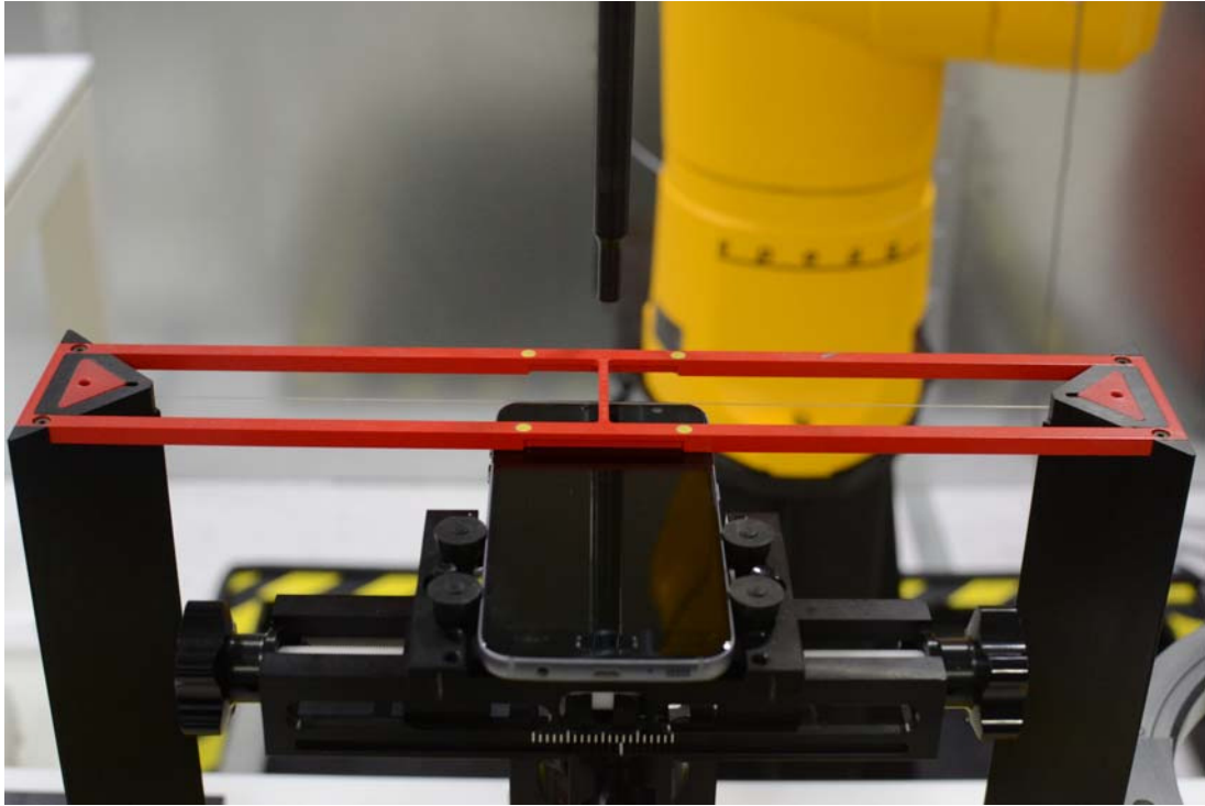
Figure 18-1 Ear Reference Point HAC Phantom Alignment
