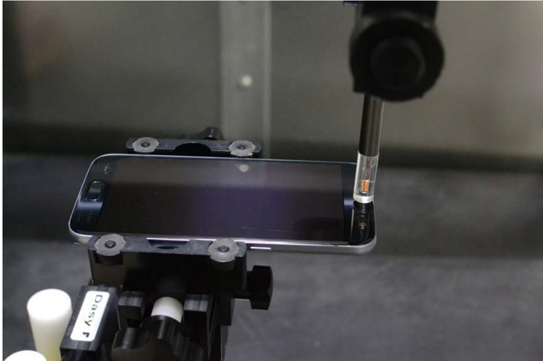
Figure 14-1 Test Setup for Wireless Device
