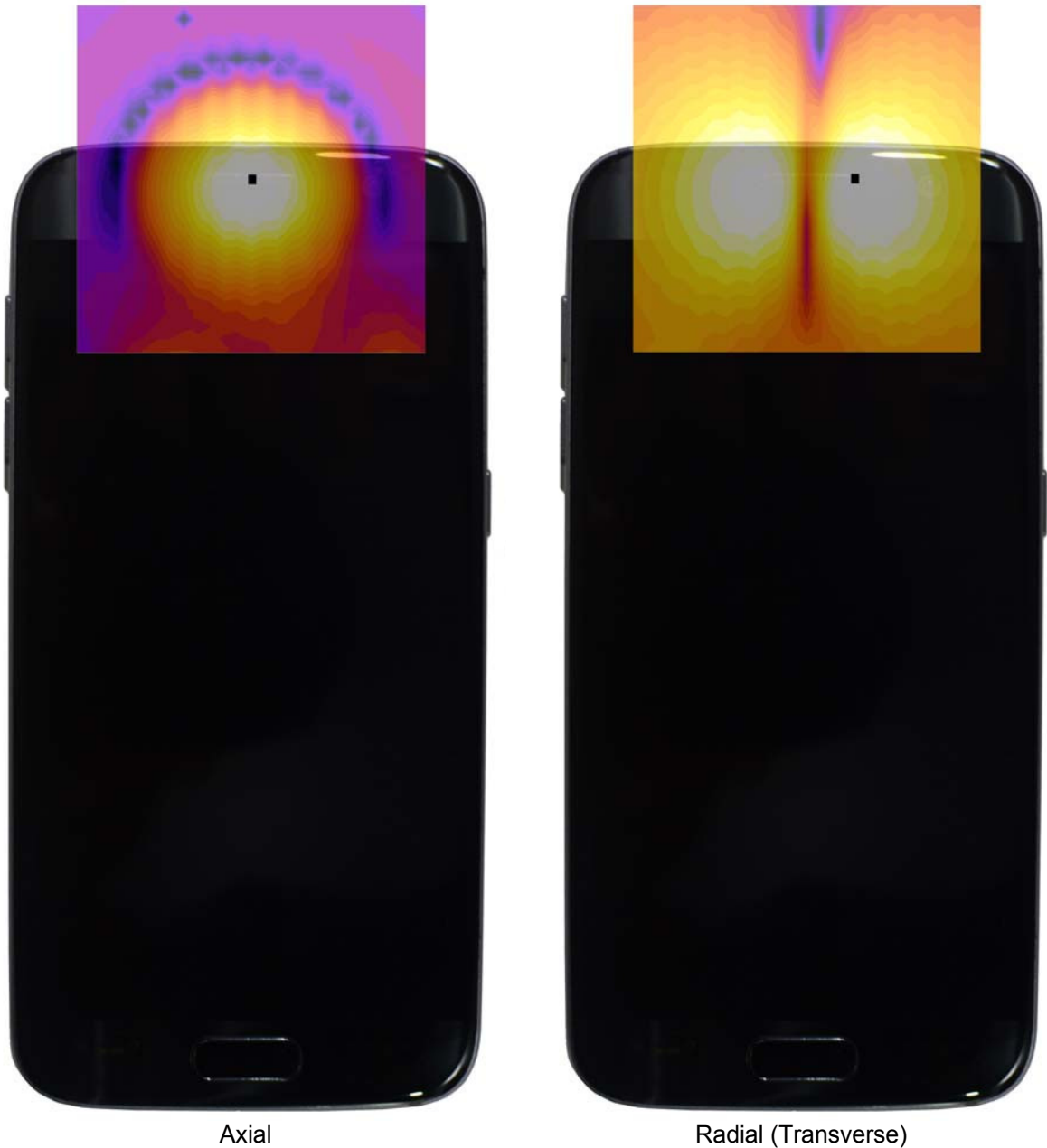
Figure 14-3 T-Coil Scan Overlay Magnetic Field Distributions
