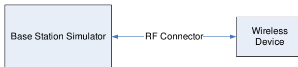
Figure 9-2 Power Measurement Setup
