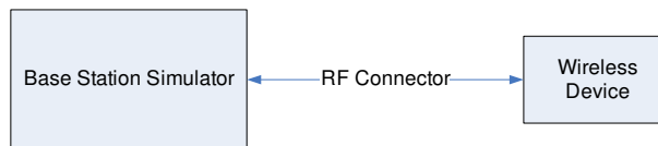
Figure 9-1 Power Measurement Setup
