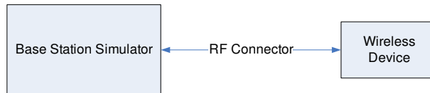
Figure 9-2 Power Measurement Setup
