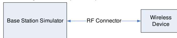
Figure 9-2 Power Measurement Setup
