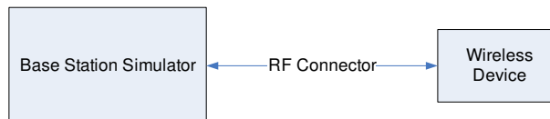
Figure 9-1 Power Measurement Setup
