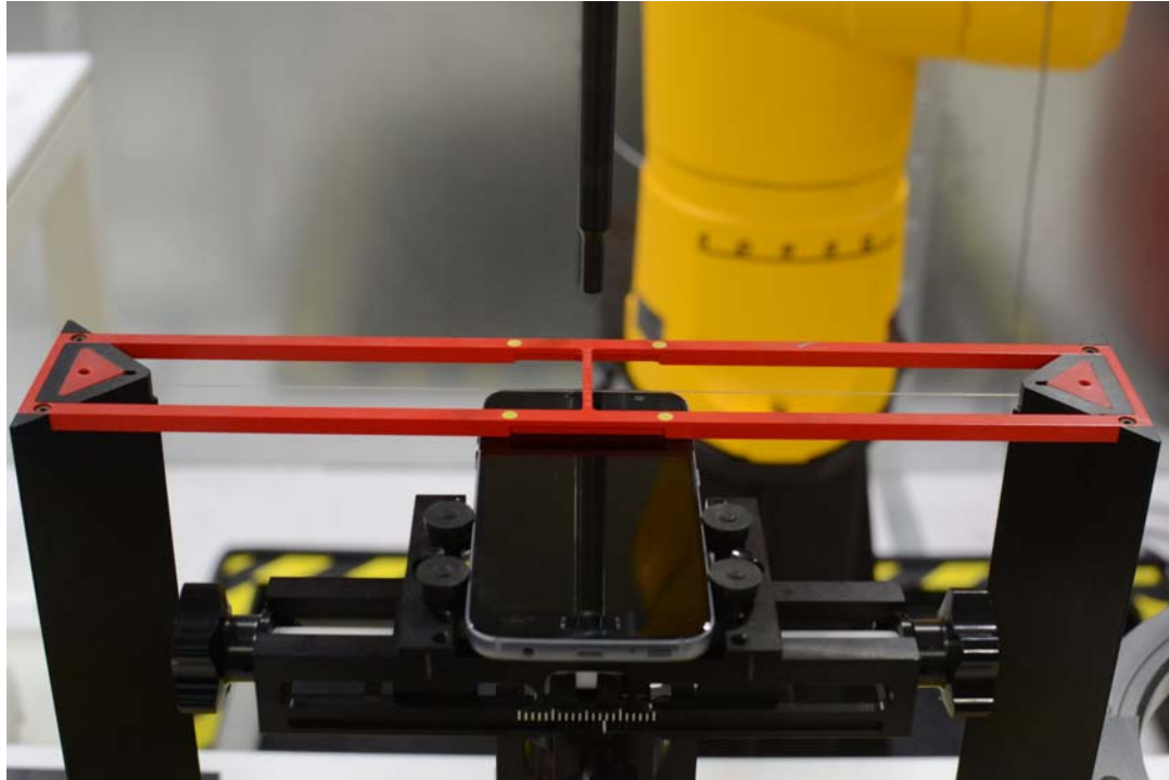
Figure 18-1 Ear Reference Point HAC Phantom Alignment
