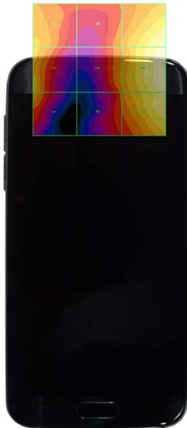
Figure 18-4 E-Field WD Scan overlay
