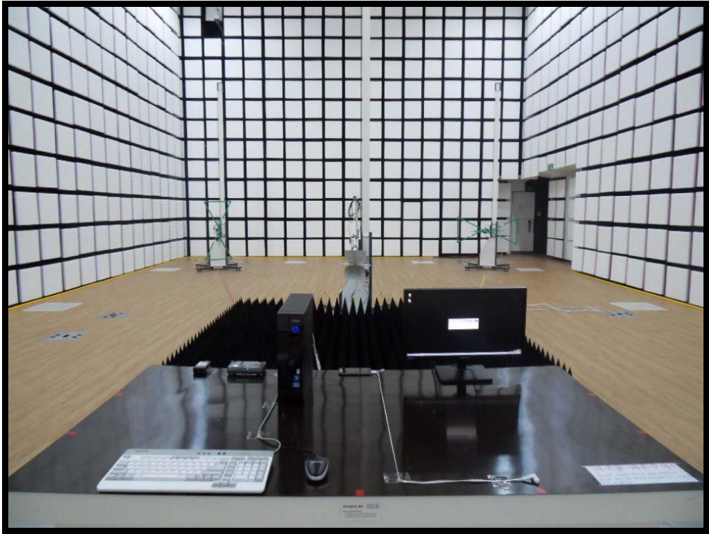
[ Radiated Disturbance for Above 1 GHz – Front ]
