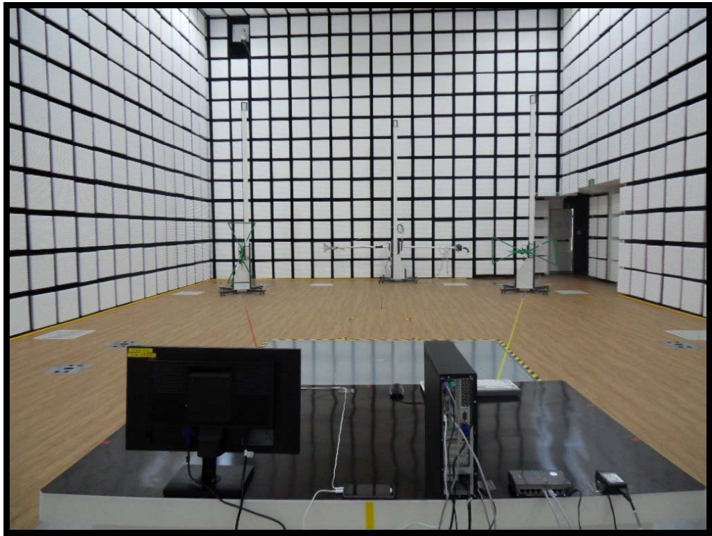
[ Radiated Disturbance for Below 1 GHz – Rear ]
