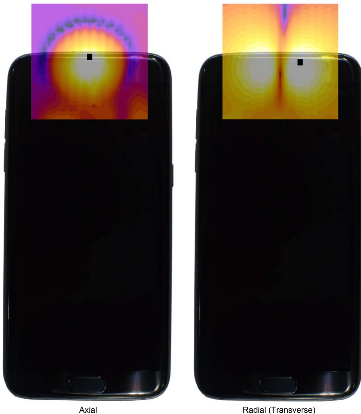
Figure 14-3 T-Coil Scan Overlay Magnetic Field Distributions
