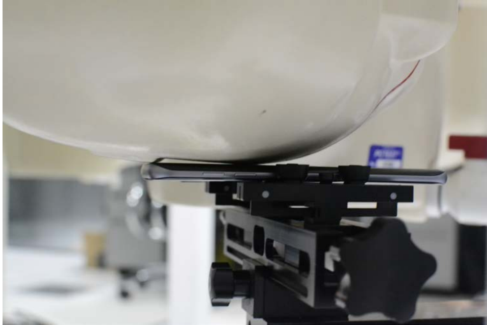
SAR Test Setup Photo 1- Right Cheek
