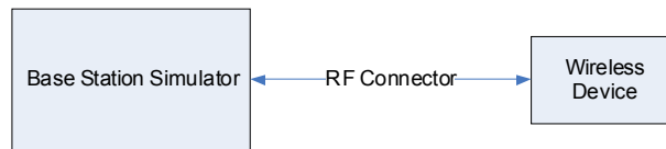
Figure 9-2 Power Measurement Setup
