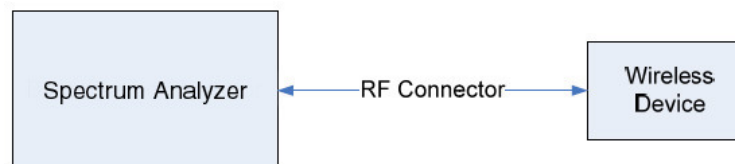
Figure 7-1. Test Instrument & Measurement Setup
