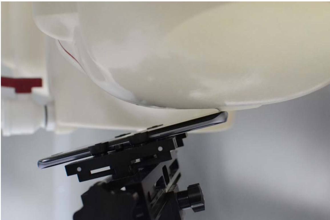
SAR Test Setup Photo 4: Left Tilt
