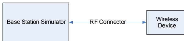
Figure 9-2 Power Measurement Setup
