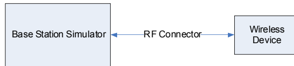
Figure 9-1 Power Measurement Setup
