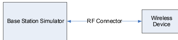
Figure 9-3 Power Measurement Setup
