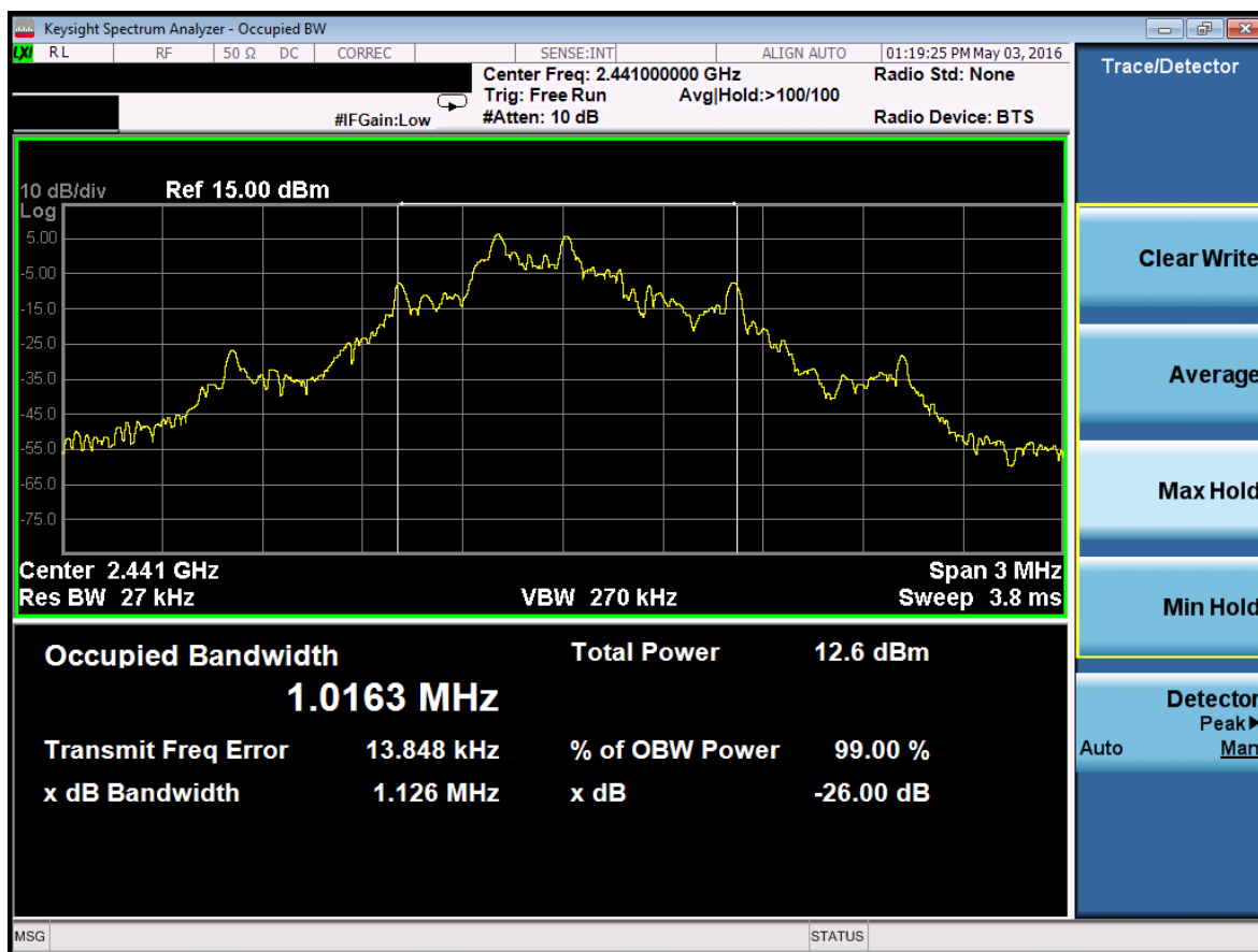
Plot 7-1. Occupied Bandwidth Plot (ANT+ – Ch. 39)
