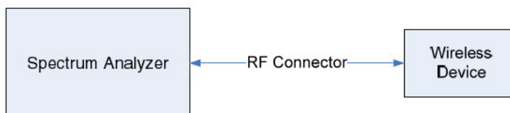
Figure 7-1. Test Instrument & Measurement Setup
