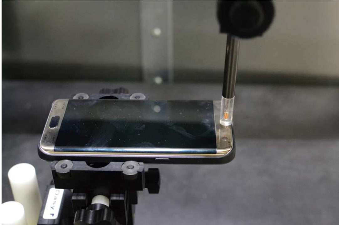
Figure 13-1 Test Setup for Wireless Device
