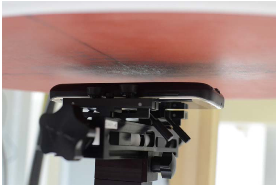
SAR Test Setup Photo 4: Back Side at 1.5 cm
